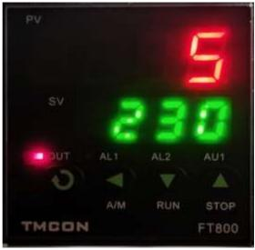
numbers) shows the preset temperature of the evaporation chamber.
